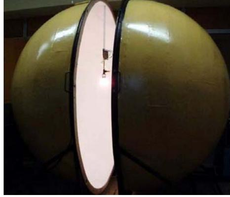
Fig. 1.2 Integrating (Ulbricht) sphere photometer.
