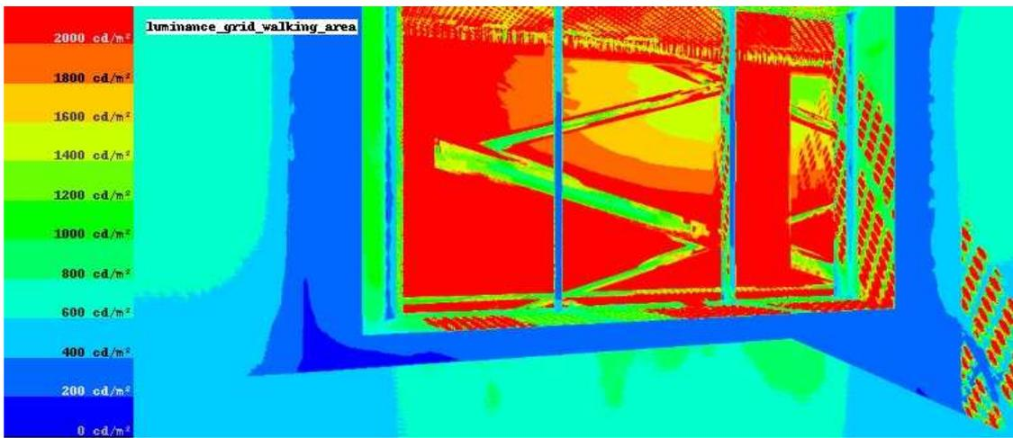
Figure 7: Images for metal grid walking area. Top: Radiance image, with luminance values for office surfaces. Bottom: False color representation of radiance image.
