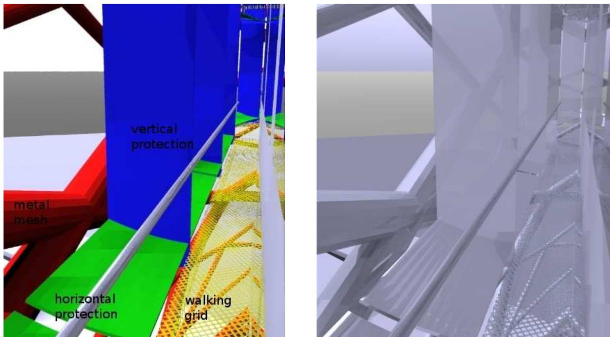
*Figure 3: Sun protections on west, south and east façade. Left image false color dummy materials and description; right image – materials used in calculations.*
