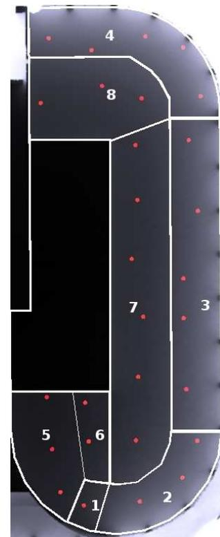
Figure 9: Position of sensor points and division of work plane into zones.
