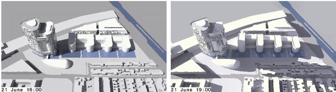
Figure 2: Shadows from tower: 21<sup>st</sup> June, 4PM (left) and 7PM (right)
