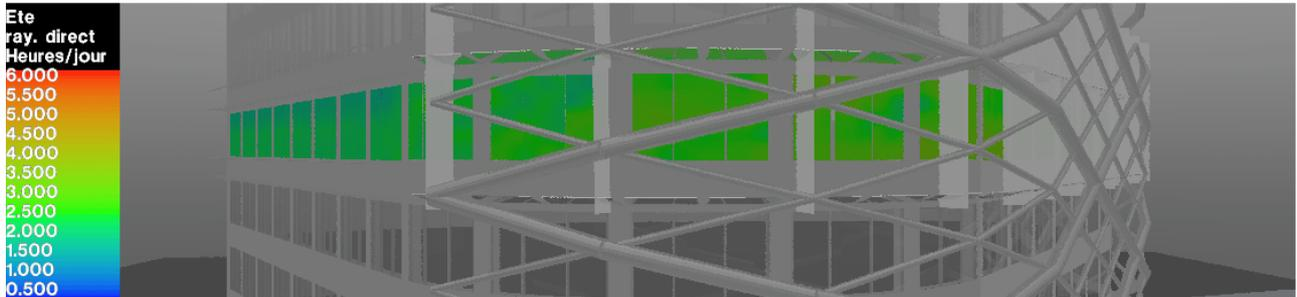
Figure 4: Average daily sun exposure for summer period without (top) and with (down) sun protections, for west part of the building. Facade on the left side of the building is oriented towards north, central curved part is west side, and right part is south facade of the building.
