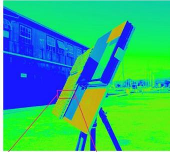
At acute angles of view, reflections from the mesh compound. The brightest reflections from the mesh will be experienced at these angles and can occur both opposite the sun and with the sun behind the viewer (retroreflection)
