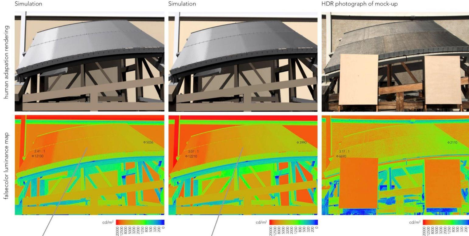
This BSDF does not have a high enough specular reflection. The ratio of left side to right side is 75% of what it should be
