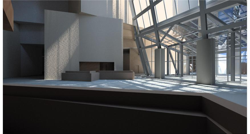
The mesh BSDF is just one of several angularly-selective transmissive materials in these views, which also include functionally-defined shade cloths and metal grating
