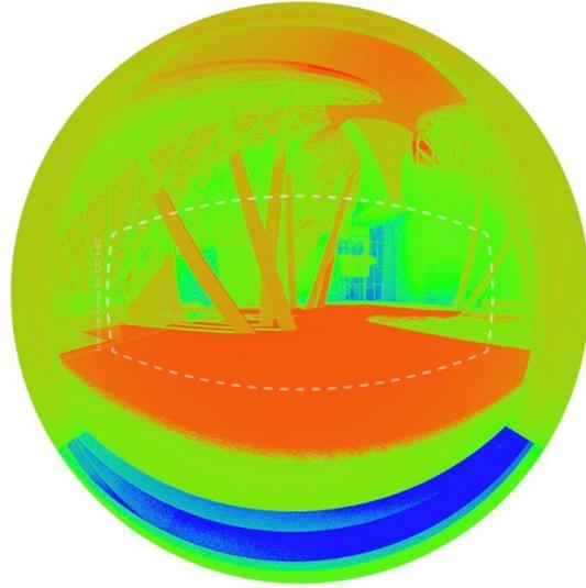
The reflections from the cone are not excessively bright and are comparably bright to the paved plaza
