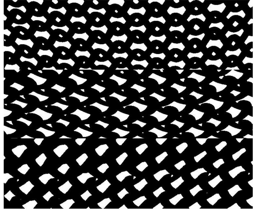
shadow projections used to calculate angular VLT of physical sample
