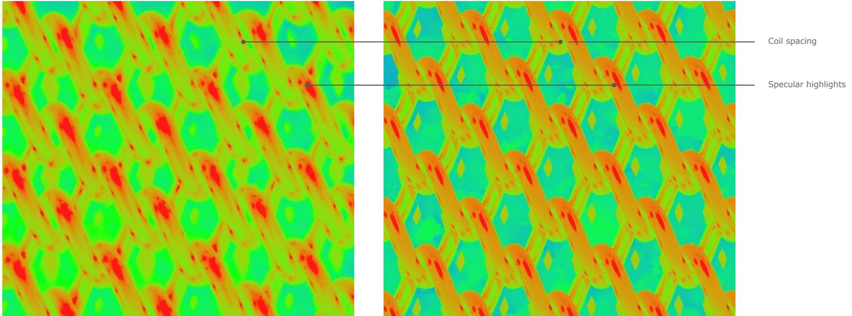
Comparisons between the physical sample (left) and simulated mesh (right) after adjustment to material and with flattening added to mesh geometry
