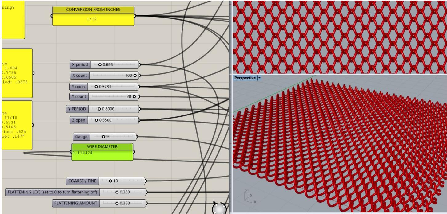
This time, we knew we would need to validate and tweak the geometry so we wrote a grasshopper script to parametrically generate the mesh.
