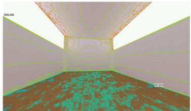
Fig. 8 False colour image of the top floor showing horizontality
