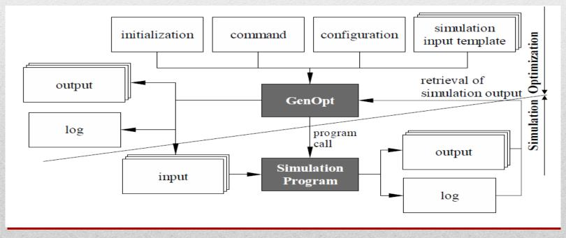
• The purpose of GENOPT (GENeral OPTimization) is to enable an engineer to create a user-friendly system of programs for analyzing and/or optimizing anything
