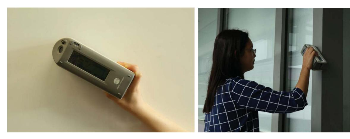
Konica Minolta 2600d spectrophotometer to measure spectral reflectance of materials
