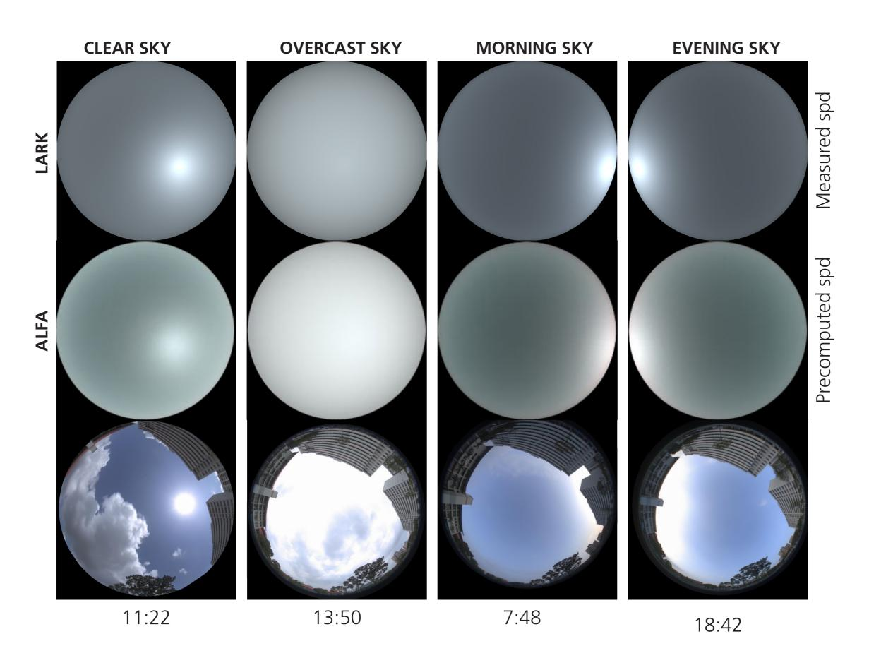
Lark uses measured global spectral irradiance and ALFA uses precomputed skies.
